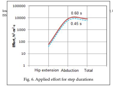
most of the effort goes into tilting the pelvis, i.e. abducting the stance hip, due to working against gravity.
